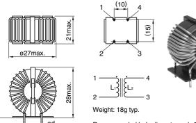
Recommended hole diameter: ød+0.5 Dimensions in mm
